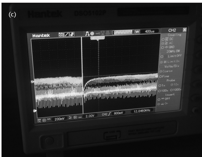
Figure 9. (a) Photograph of a plasmon-polariton wave along a wire. (b) Current and voltage along the wire on the oscilloscope screen. The oscillation has an increasing amplitude only in hydrogen. It has a steady amplitude in air. The spark gap is driven by relaxation oscillator, that is, discharging a capacitor. (c) Note gradual increment of the voltage oscillations (above) and current oscillations (below).
