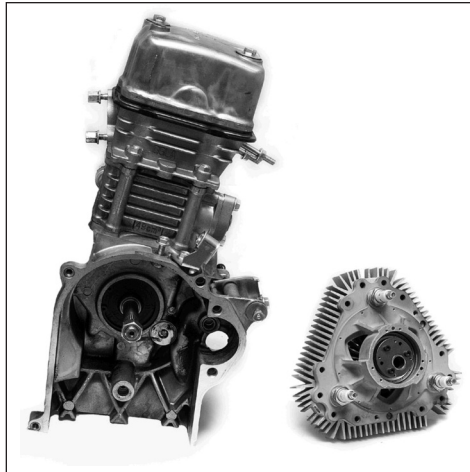
Figure 1. Comparing a rotary internal combustion engine to the usual piston and crankshaft type 4 stroke engine of the same power. The power density is 1:10!
