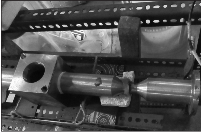
Figure 4. Suhas Ralka's ultrasound driven fuel preparation device based on watery tungsten sludge. Note the three sonotrodes, the sound conductors. They conduct the ultrasound waves to the treated sludge.
